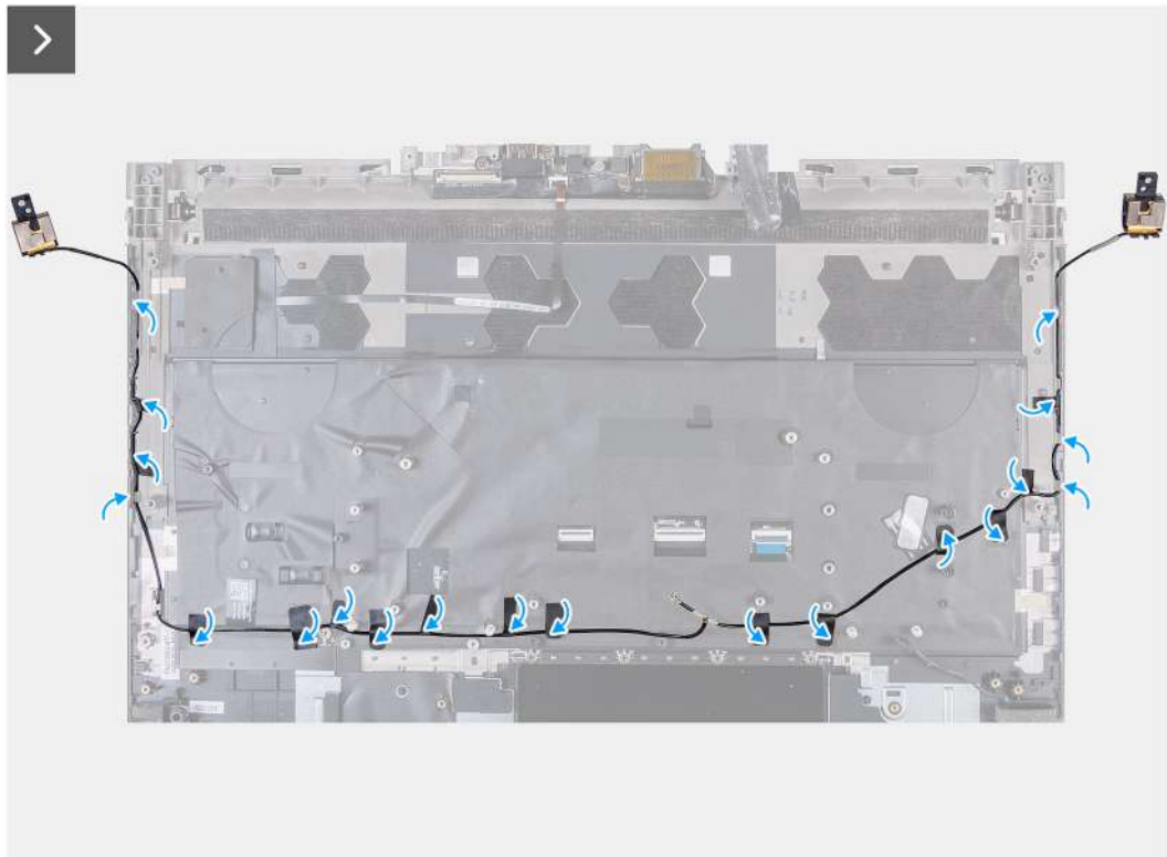
Figure 47. Installing the antennas
