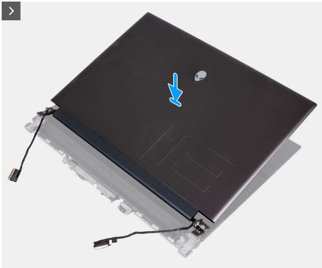
Figure 38. Installing the display assembly
