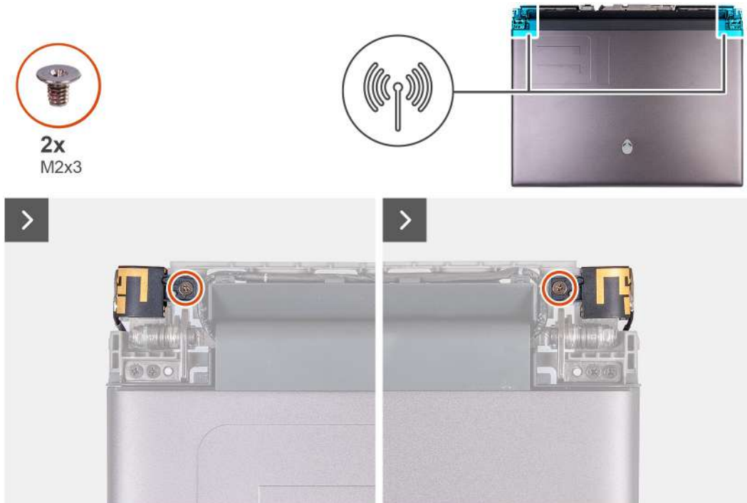
Figure 46. Removing the antenna
