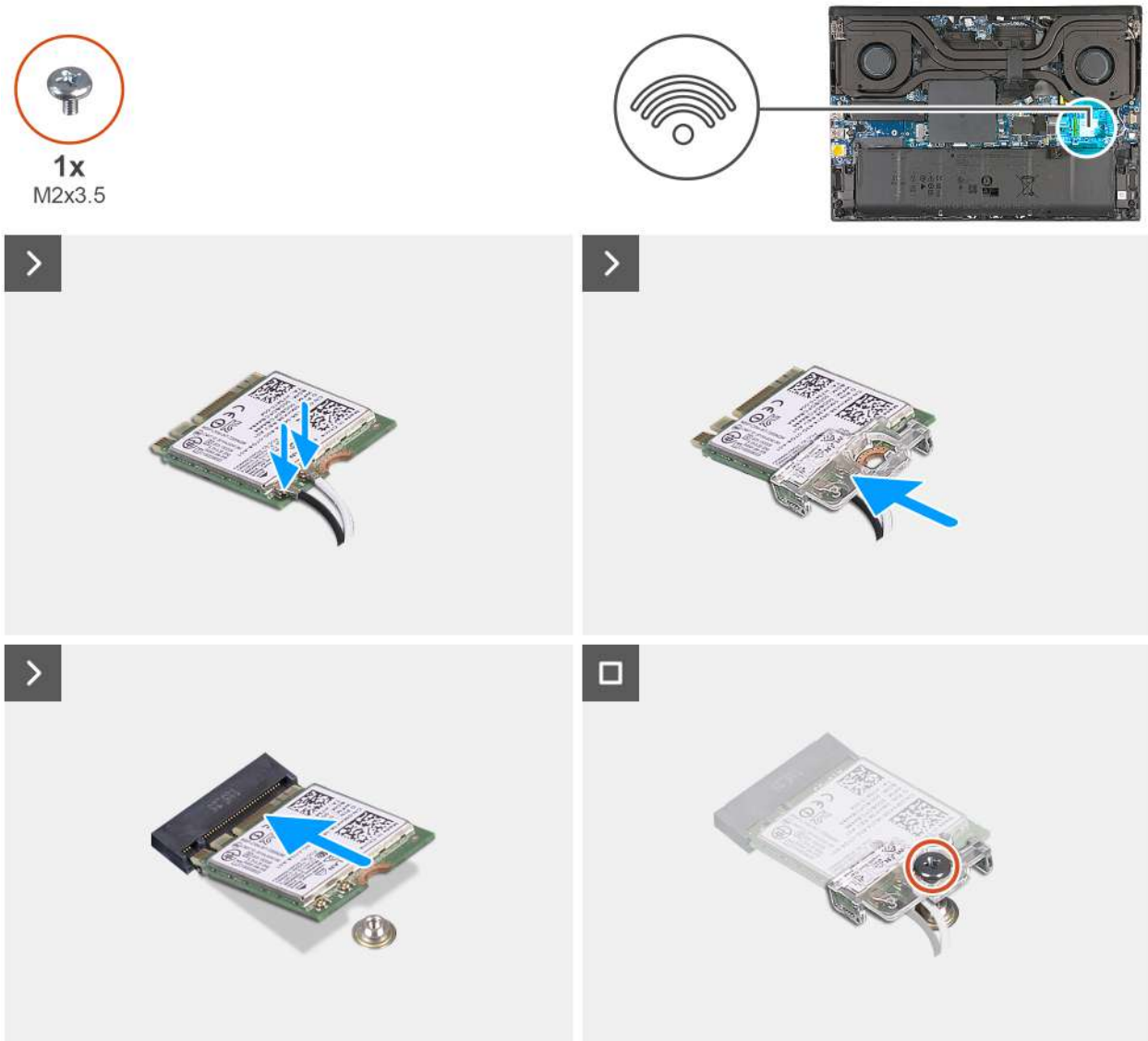
Figure 18. Installing the wireless card
