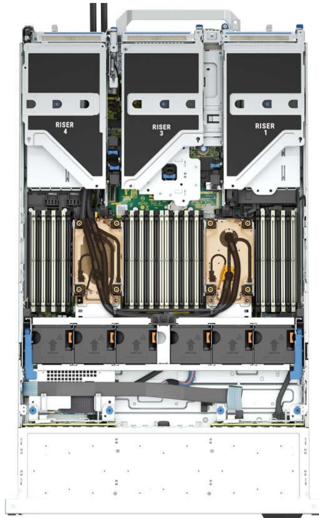
Figure 11. Inside the system with processor liquid cooling module
