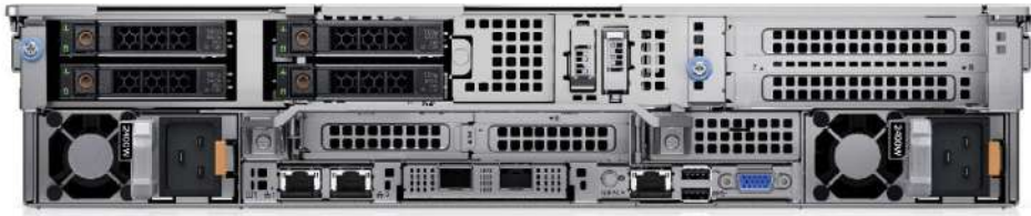
Figure 12. Rear view of the R750 with 4x 2.5 inches storage drives, 4x PCIe Gen4 slot and Hot-plug BOSS
