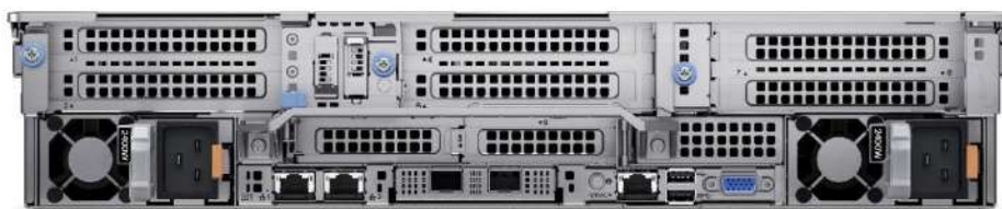
Figure 11. Rear view of the R750 with 8x PCIe Gen4 slots and Hot-plug BOSS
