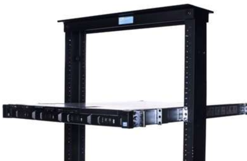
Figure 19. System mounted in static rails in two-post center-mount configuration
